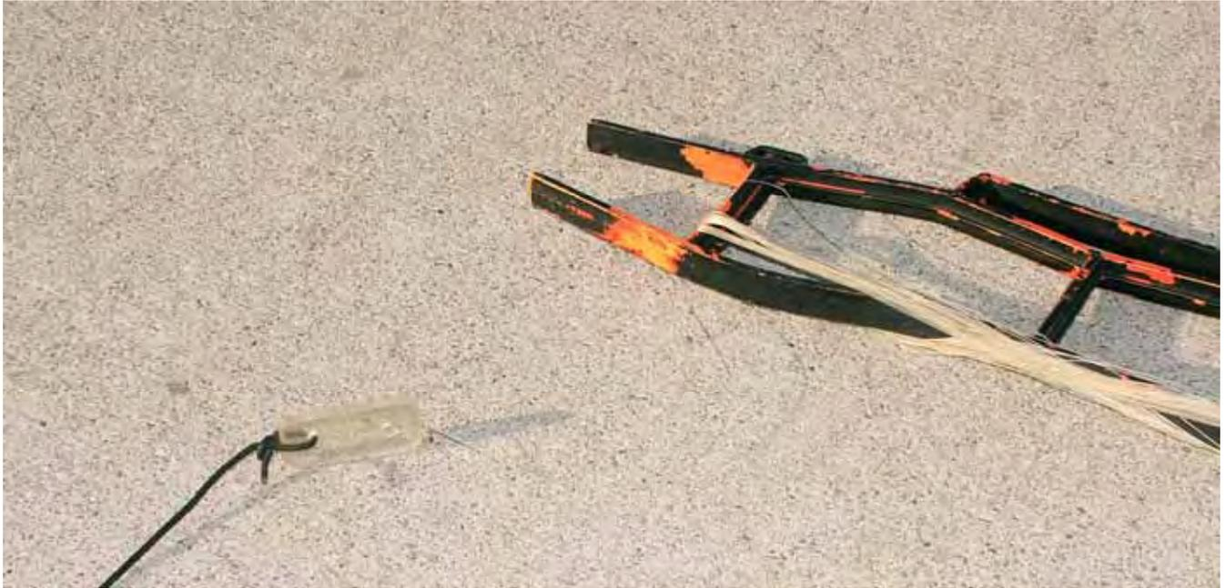
If black zip cord is used, and the insulators and winders are painted flat black, the antenna is mostly “invisible” in a campground. Highly visible flagging should be attached for safety, if necessary.
