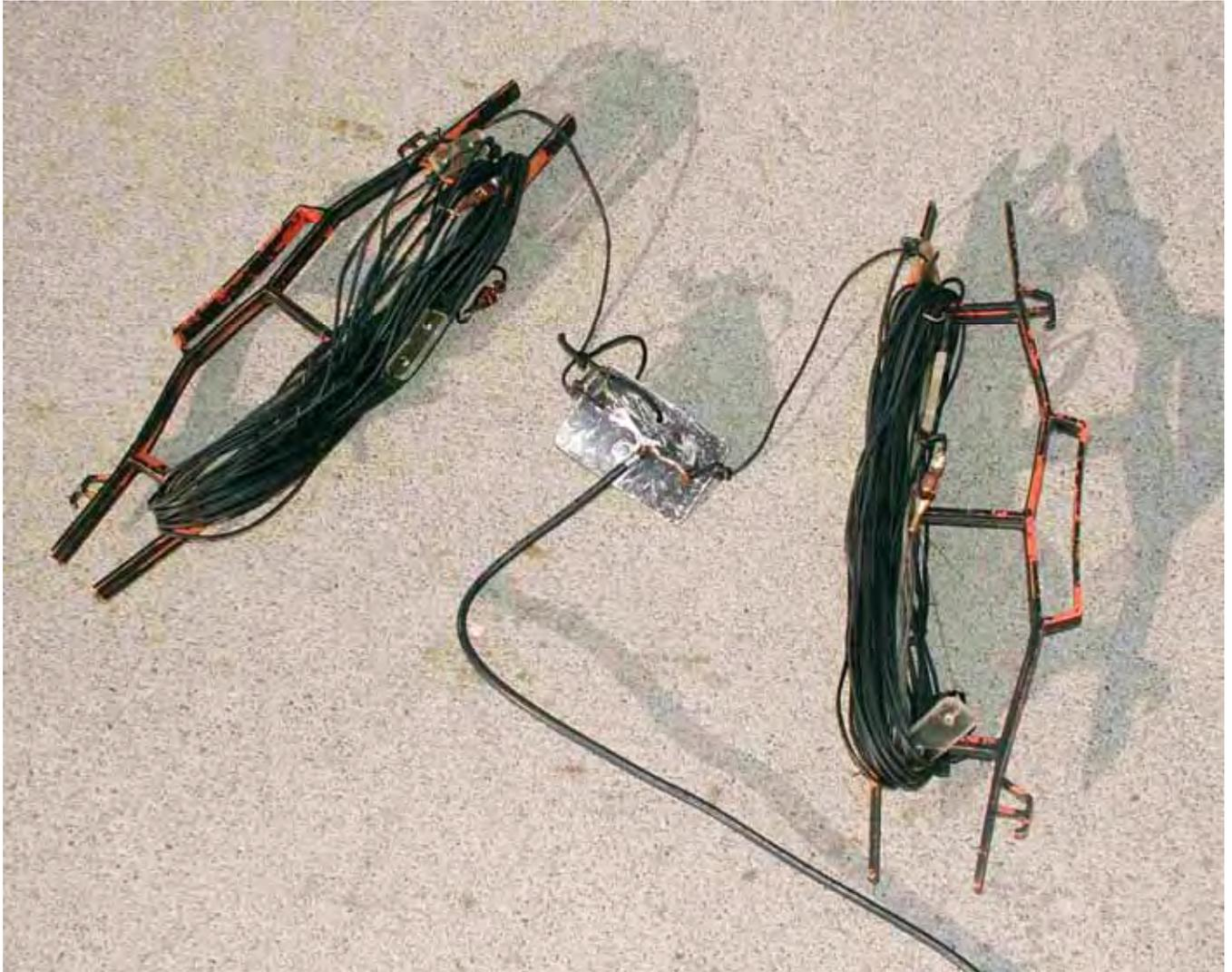
The need for an “all band” portable antenna which performs well, and is easy to use, led to the development of the following wire antenna. It works, without needing a tuner, on the 80, 75, 40, 30, and 20 meter bands.
