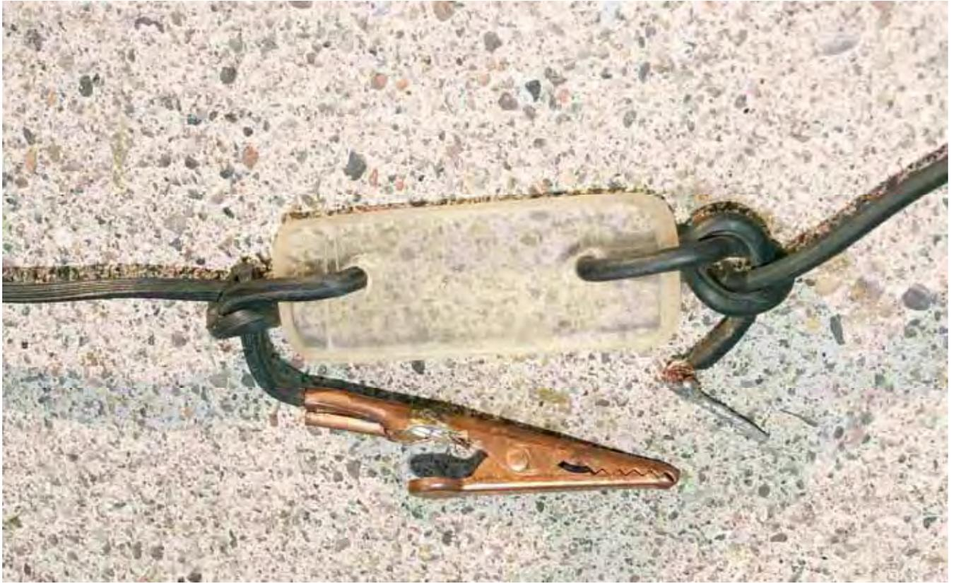
Each length of each segment is measured, cut, and installed sequentially; resulting in the following lengths from the middle of the center insulator to the MIDDLE of each insulator. Allow about 1 extra inch of wire for the securing knot.
