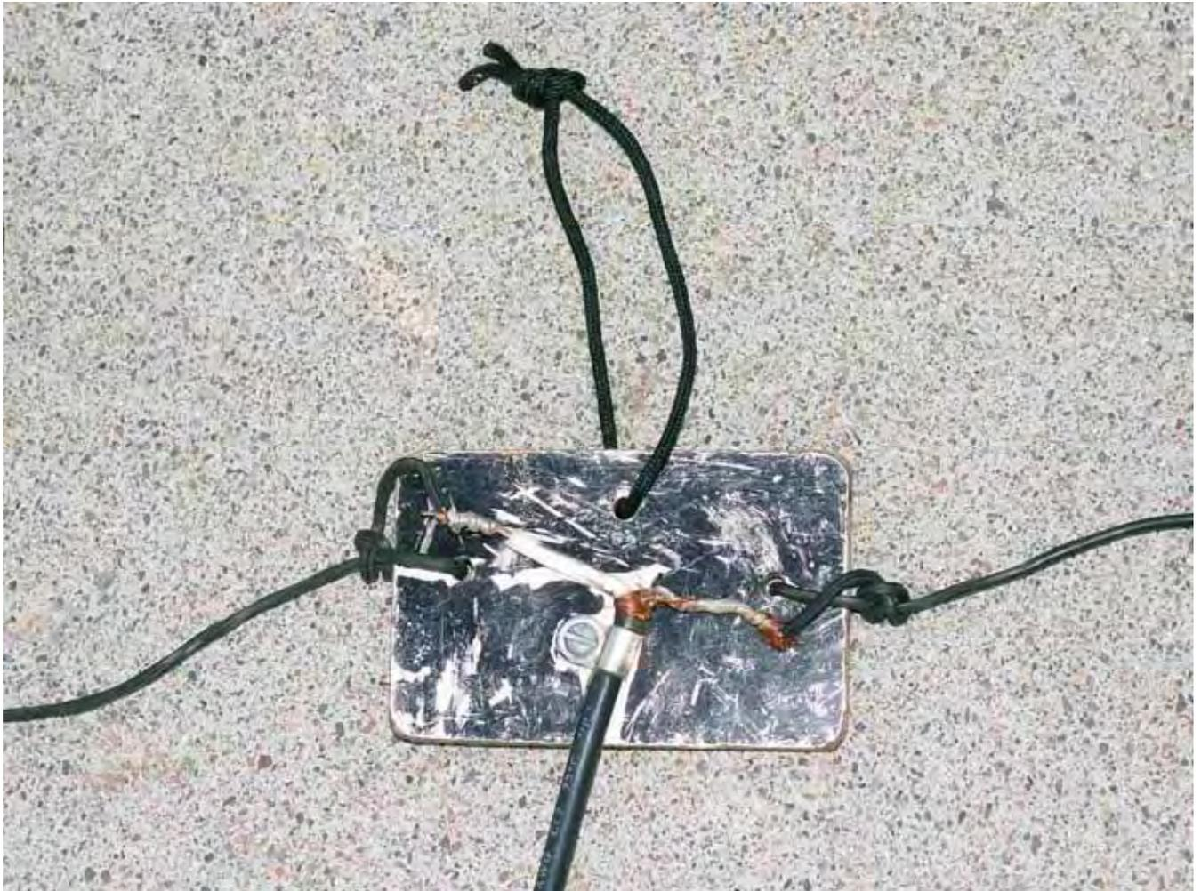
The center insulator is a piece of 1/8 inch thick masonite, approximately 5 x 3 inches. The coax is attached to the center insulator with a small metal clamp, bolted to the insulator. Each side of the antenna is looped through a hole drilled in the insulator, and secured with a knot. All connections are soldered.
